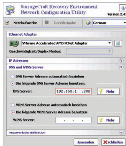
Figure 3: In the boot CD network tool, the administrator may enter a DNS and a WINS server independently of the DHCP.
